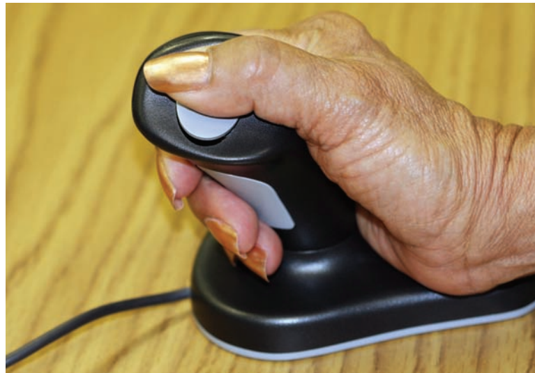
A joystick “mouse” that can be used by those with limited dexterity. Very little pressure is needed for left or right clicking.
